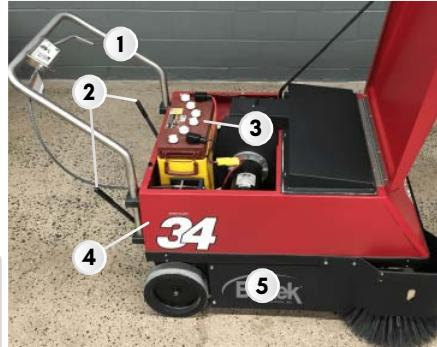
No matter what you need to tackle, the Factory Cat 34 is able to handle your heavy-duty cleaning needs. Easily pick up metal shavings, foundry sand, woodchips, broken glass, paper, dirt and dust. In fact, this walk-behind sweeper can sweep up multiple bags of cement without leaving any dust behind or blowing it into the air, thanks to its polypropylene felt "baghouse" filter. Because the filter is cleaned by an on-board mechanism, it typically lasts the length of the machine.
