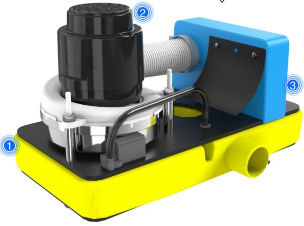
3 Blue Reservoir: Designed to muffle the vacuum exhaust as well as serve as a check point during cleanings, the reservoir empties into a clear catch. By monitoring you can ensure proper usage.
