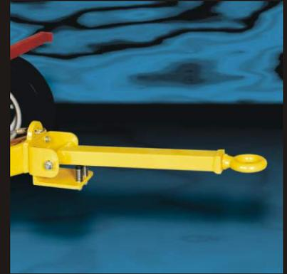
*The self-leveling tongue increases operator efficiency and performance by maintaining the trailer tongue at the precise height for hook-up.*
