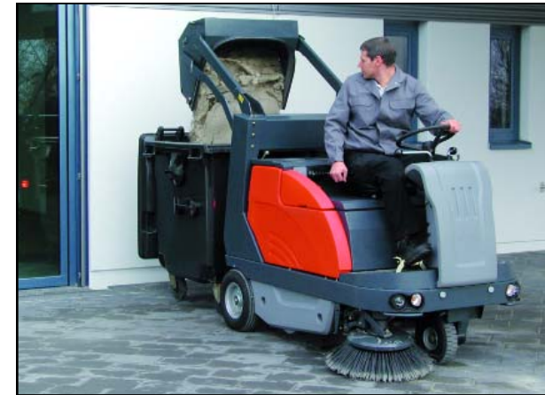
The high dump hopper can be easily emptied into large containers.
