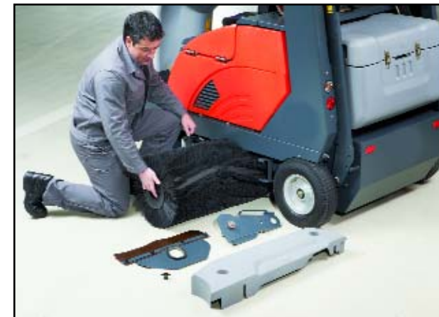
Change-out of main sweeping brush requires no tools and is quick and simple.
