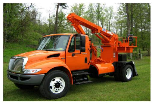
Ramer Shuttle Loader system allows the loader to remain on the job loading other trailers while the loaded trailer is "shuttled" by another truck to the dump site.
