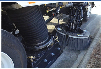
VACUUM AND BRUSH REMOVAL OF DEBRIS
