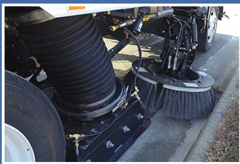
VACUUM AND BRUSH REMOVAL OF DEBRIS
