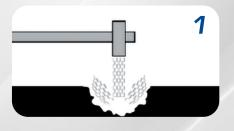
Cleaning – Dust and debris is blown from the pothole by a high velocity blower. The Operator is located in the cab eliminating being exposed to traffic and reducing the risk of potential personal injury.
