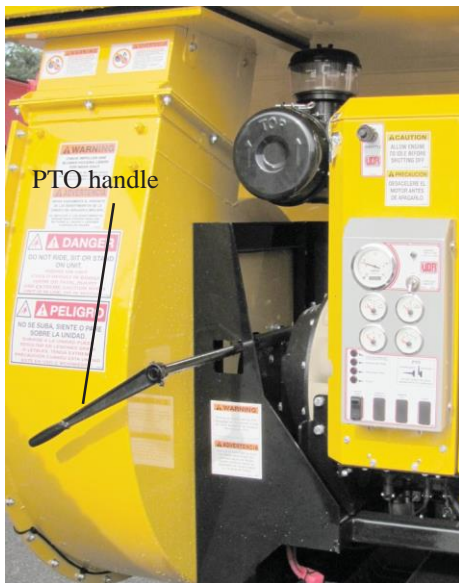
PTO shown disengaged
