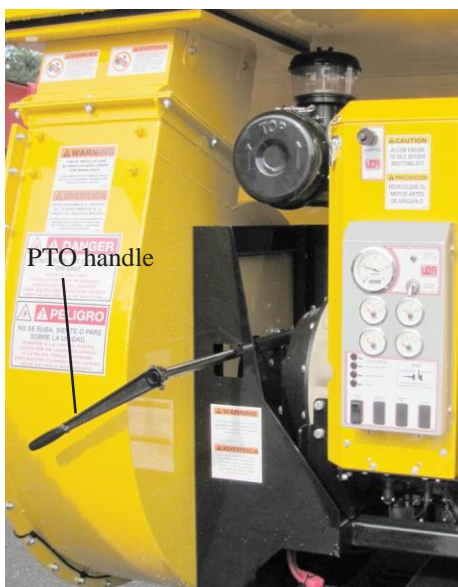
PTO shown disengaged
