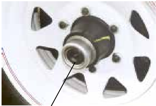
Grease fitting is behind rubber plug
