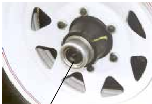
Grease fitting is behind rubber plug
