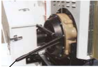
PTO shown disengaged
