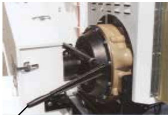
PTO shown disengaged
