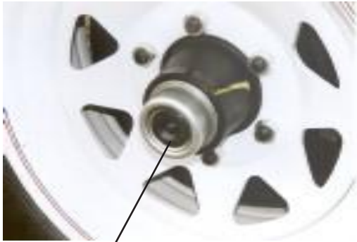
Grease fitting is behind rubber plug
